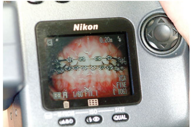
Figure 13 Focal length set at 0.2 m (top right), camera moved until image sharp
