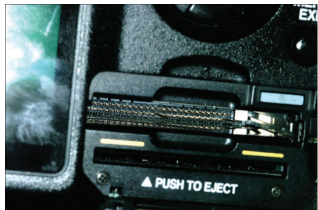
Figure 21 Damaged card bends the pins inside the camera
