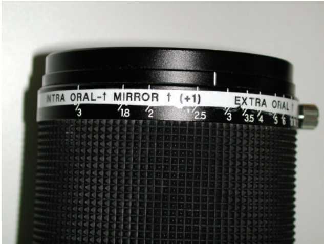
Figure 1 Fixing the focal distance ensures consistent magnification
